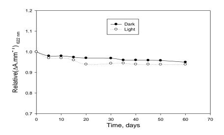
Fig. 5. Post-irradiation stability of (BTB-MO)/ PVA films stored under different storage conditions.
