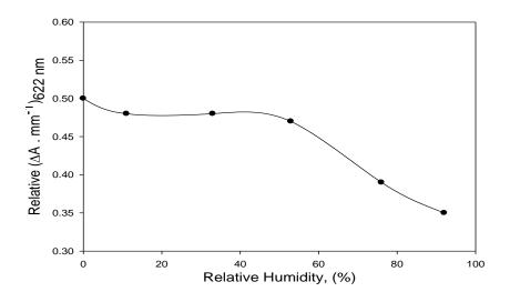
Fig. 4. Variation of response of (BTB-MO)/ PVA films (at 622 nm) as a function of relative humidity during irradiation, where response in ∆A. mm-1 at 30 kGy.
