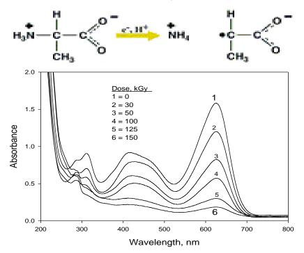
Fig. 2. The absorption spectra of (BTB-MO)/ PVA films unirradiated and irradiated to different absorbed doses. [α-alanine]= 66.6 phr.
