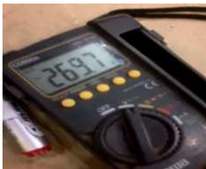
Fig.18. Output voltage of the two inverters by voltammeter at no load.
