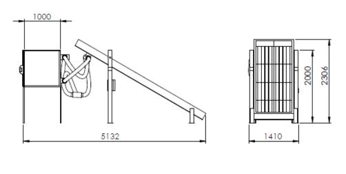
Left ViewFront View1: solar collector2: drying chamber3: blowerFig. (1): Isometric, top, left and front view for the solar dryer.
