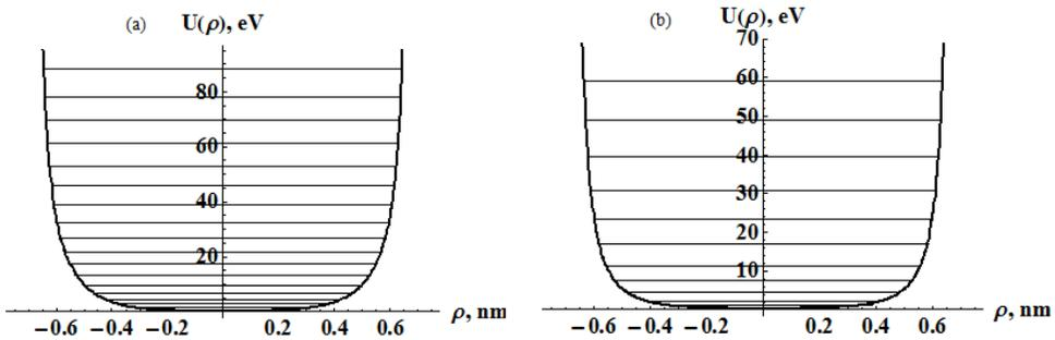
**Fig. (4):** Channeling potential of positrons channeled in an (10,10) single wall carbon nanotube as a function of a distance  $\rho$  from the center of the tube in a plane normal to the tube axis, (a) Moliere atomic potential, (b) Universal atomic potential. Some eigenvalues of 100 MeV positrons incident in the direction parallel to the nanotube axis are shown by horizontal lines.
