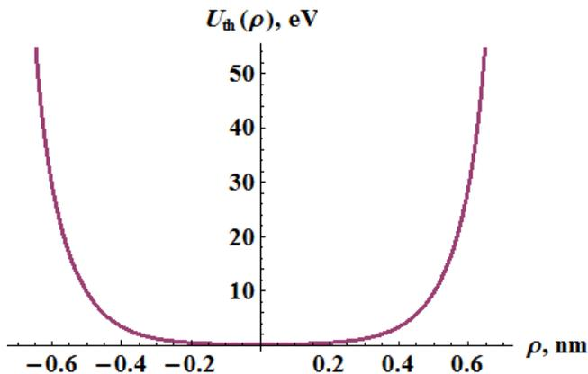
**Fig. (3):** Channeling potential of positrons channeled in (11,9) single wall carbon nanotube as a function of a distance  $\rho$  from the center of the tube in a plane normal to the tube axis. The curve represents the present work by using Moliere atomic potential and the potential as given in Ref. [14]. The calculations is executed at thermal vibration amplitude  $u_l = 0.0053 \text{ nm}$ .
