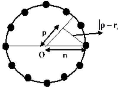
**Fig. (1):** Cross section of the nanotube channel is a circle of radius  $r$ , the rows of the carbon atoms are positioned at  $\mathbf{r}_i$  over the circumference of the nanotube,  $\boldsymbol{\rho}$  the distance from the nanotube center.
