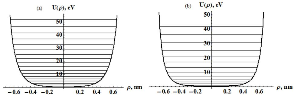
**Fig. (5):** Channeling potential of positrons channeled in an (11,9) single wall carbon nanotube as a function of a distance  $\rho$  from the center of the tube in a plane normal to the tube axis, (a) Moliere atomic potential, (b) Universal atomic potential. Some eigenvalues of 100 MeV positrons incident in the direction parallel to the nanotube axis are shown by horizontal lines.
