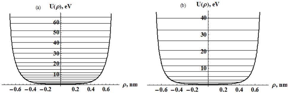
**Fig. (6):** Channeling potential of positrons channeled in an (18,0) single wall carbon nanotube as a function of a distance  $\rho$  from the center of the tube in a plane normal to the tube axis, (a) Moliere atomic potential, (b) Universal atomic potential. Some eigenvalues of 100 MeV positrons incident in the direction parallel to the nanotube axis are shown by horizontal lines.
