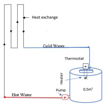
Figure (4): The electrical heating system.
