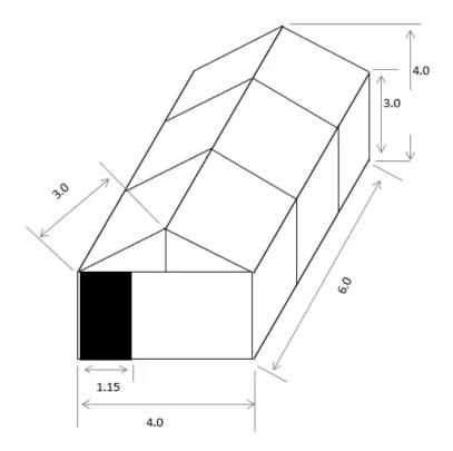
Figure (2): The schematic diagram of gable-even-span greenhouse.
