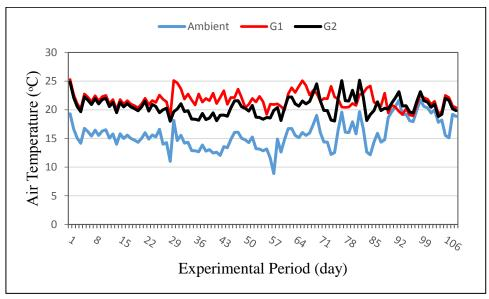
Figure (5): The daily average air temperatures diurnal changes in temperatures of the air inside and outside the greenhouses.
