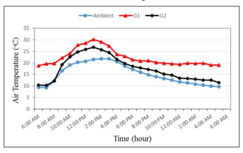
Figure (6): The hourly average air temperatures inside and outside the greenhouses.
