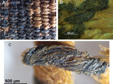
Fig. 4. UV-VIS miceroscope images of (a, b, c) textile samples painted with carbon charcoal. The images show cleary the mask and deposition of the particles on and in-between the fibre surfaces.
