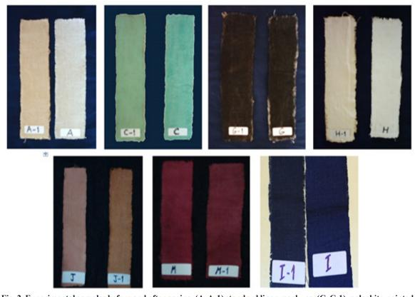
Fig. 2. Experimental samples before and after ageing, (A, A-1) standard linen mockups, (C, C-1) malachite-painted mockups, (G, G-1) charcoal-painted mockups, (H, H-1) Calcite-painted mockups, (J, J-1) madder-dyed mockups, (M, M-1) cochineal-dyed mockups, (I, I-1) indigo-dyed mockups.
