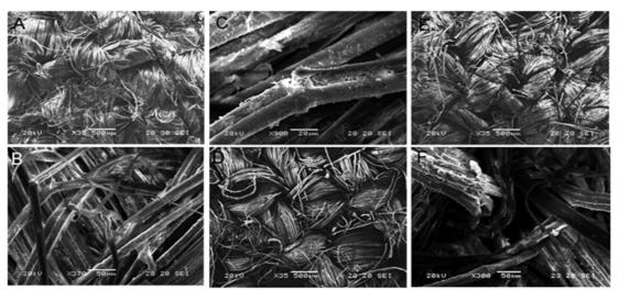
Fig. 6. SEM microphotographs of the dyed textile samples with (a, b) indigo, (c, d) madder, (e, f) cochineal, show that the dye molecules are small enough to penterate into the fibres without changing the fibre morphology. Also show minor degredation of the linen fiber surface after thermal ageing as small scratches and longitudinal splitting.
