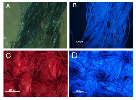
Fig. 3. UV-VIS miceroscope images of (a, b) fiber samples dyed with indigo dye, (c, d) Cochineal-dyed sample.
