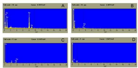
Fig. 7. EDX results of the experimental coloured textile fibres with (a) malachite, (b) black charcoal, (c) calcite and (d) madder.
