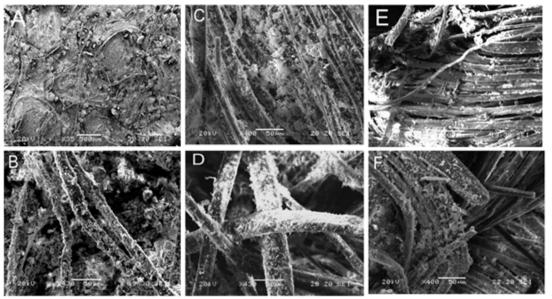
Fig. 5. SEM microphotographs of the painted textile samples with (a, b) malachite, (c, d) calcite, (e, f) black charcoal. The images illustrate the deposition of pigments particles on and in-between the fibers.
