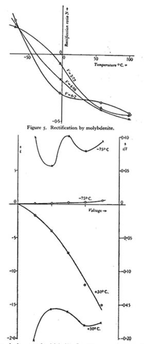
Figure 6. A.-c. test of molybdenite. O, current; ×, current ratio N.
