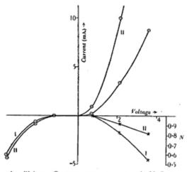
ugure 3. Rectification by silicium.  $\odot$ , current; x, current ratio N; I at  $-75^{\circ}$  c.; II at  $+30^{\circ}$  c.
