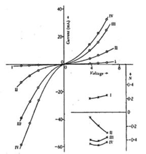
Figure 4. Change of sign of rectification by molybdenite.  $\odot$ , current;  $\times$ , current ratio N; I at  $-70^{\circ}$  c.; II at  $-3^{\circ}$  c.; III at  $+58^{\circ}$  c.; IV at  $+100^{\circ}$  c.
