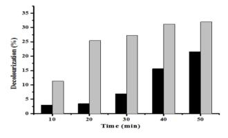
Fig. 7. The decolourization (%) of  $3 \times 10^{-5}$  M RR by 0.08g [(Fe<sub>3</sub>O<sub>4</sub>/PAAc/PVA)/TiO<sub>2</sub>] PAAc, temperature (30±0.1 °C) and pH 6.8.
