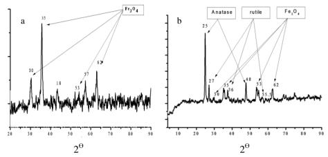
Fig. 1. XRD pattern: a) Fe<sub>3</sub>O<sub>4</sub>/PVA/PAAc & b) [(Fe<sub>3</sub>O<sub>4</sub>/PAAc/ PVA)/TiO<sub>2</sub>] PAAc.
