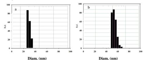
Fig. 3. Particle distribution: a) Fe<sub>3</sub>O<sub>4</sub>/PAAc/ PVA powders & b) [(Fe<sub>3</sub>O<sub>4</sub>/PAAc/ PVA)/TiO<sub>2</sub>] PAAc.
