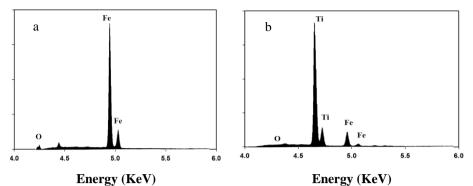
Fig. 2. EDX spectrum: a) Fe<sub>3</sub>O<sub>4</sub>/PVA/PAAc & b) [(Fe<sub>3</sub>O<sub>4</sub>/PAAc/ PVA)/TiO<sub>2</sub>] PAAc.
