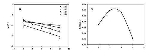
$\begin{array}{ccc} & & & pH \\ \hline \label{eq:Fig. 8. catalytic degradation of 3×10-5M RR at a) Influence of pH on 0.08g \\ [(Fe_3O_4/PAAc/ PVA)/TiO_2] PAAc and temperature (30\pm0.1 \circ C). b) \\ & Variation of rate constant K (min<sup>-1</sup>) with different pH at concentration \\ & 3\times10^{-5} \ M \ of \ RR \ with \ 0.08 \ g \ [(Fe_3O_4/PAAc/ PVA)/TiO_2] \ PAAc \ and \ temp \\ & (30\pm0.1 \circ C). \end{array}$
