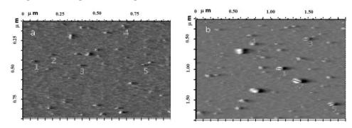
Fig. 5. Topographical scans for the surface: a) Fe<sub>3</sub>O<sub>4</sub>/PAAc/ PVA & b)  $[(Fe_3O_4/PAAc/ PVA)/TiO_2]$  PAAc.
