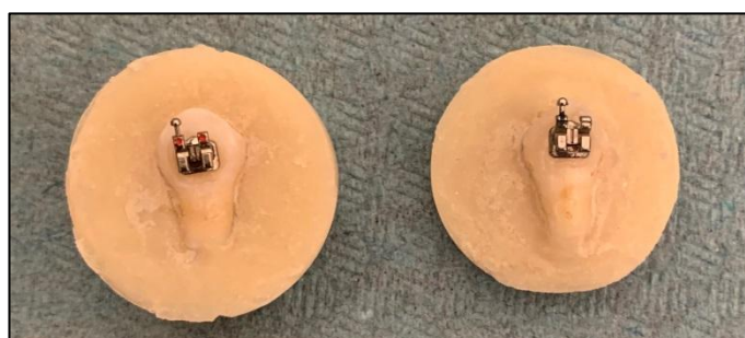
Figure 1: Brackets bonded and mounted in acrylic mold.
