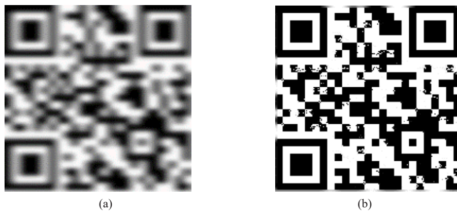
Fig. 6: (a) Distorted Image6 by a 2.0 pixels radius Gaussian blur followed by a distance of 10 pixels motion blur (b) PAF.
