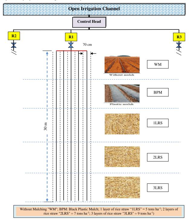
Figure (2): Layout of the experimental design.
