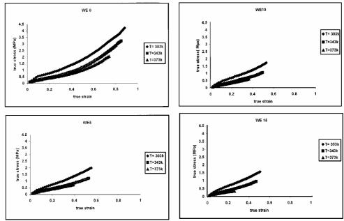
Fig. (1) True stress vs true strain under extension at, 30°C, 70°C and 100°C, for samples W0, W5, W10 and W15.
