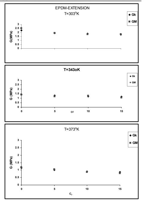
Fig. (5) The variation of  $G_k$  and  $G_M$  as a function of foaming agent concentration,  $C_f$ , at different temperature 30, 70 and 100 °C respectively under extension.
