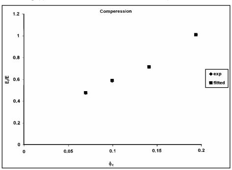
Fig. (9) The variation of the relative modulus,  $E_{f'}\!E_{VS}\,\phi_C$  in comperession.
