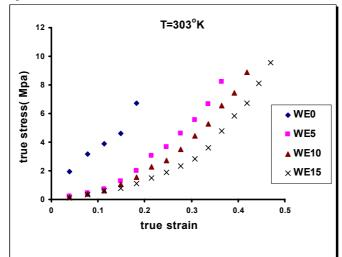
Fig. (2) True stress vs true strain under compression at, 30°C for the investigated samples.
