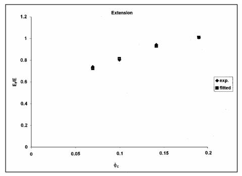
Fig. (8) The variation of the relative modulus,  $E_{f}\!/E_{VS}\,\phi_{C}$  in extension.
