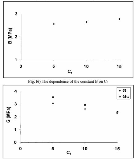
Fig. (7) The variation of G as a function of foaming agent concentration,  $C_f$ , at 30 °X υνδερ χομπρεσσιον.
