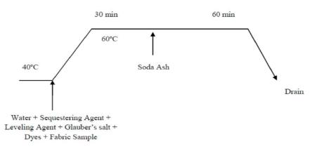
Fig. 3. Dyeing procedure curve
