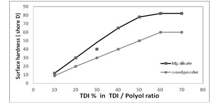
Fig. 3. Effect of TDI percent in TDI / polyol ratio on surface hardness of PUmodelling clay.
