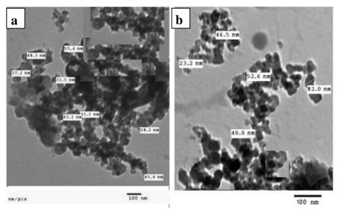
Fig. 3. TEM images of (a) CS50VC and (b) CS100VC. Scavenging Activity (%)
