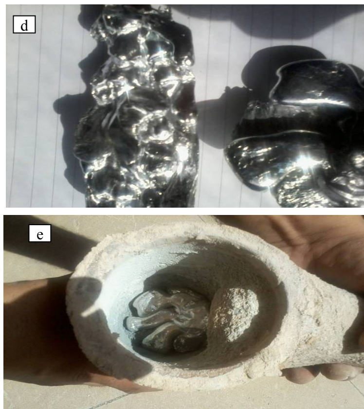
Fig. 2. A photograph of the pyrometallurgical system used for Zn recovery and recovered zinc from Zn-dross.
