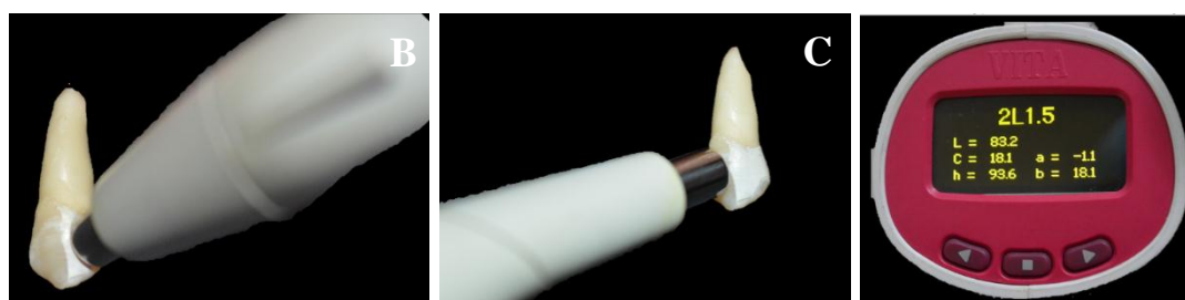
Fig (3): A: spectrophotometer measuring right buccal surface of each specimen on which the WSL was formed B: spectrophotometer measuring left buccal surface of each specimen. C: the analysis displayed on the spectrophotometer screen giving the components of color L^* , a^* , and b^* .
