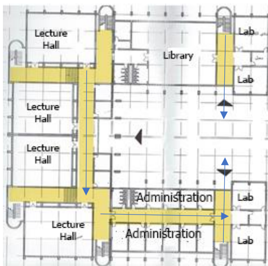
Figure 4: The use of two exits only on the ground floor and the closure of the middle exit in a way that does not meet the requirements of the exit discharge. [4]
