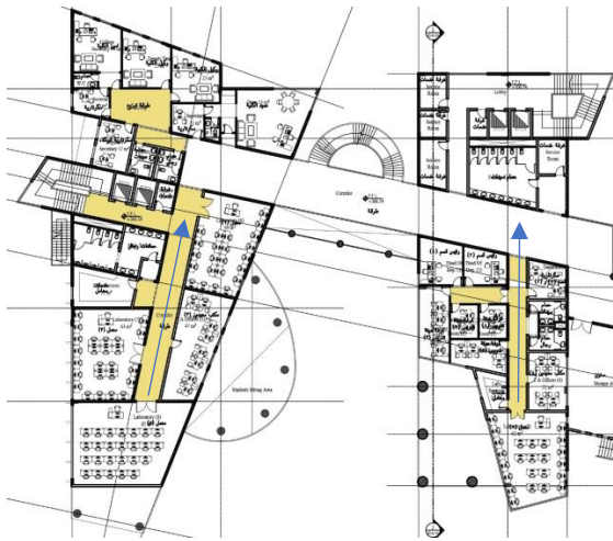
Figure 15: The distances of the dead ends, which is 20 meters in some areas. [5]
