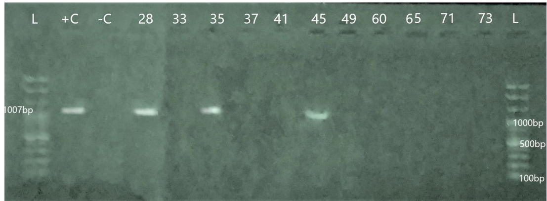
Fig. 1. Gel photo for bla SHV gene in E. coli isolates from the two WWTPs [L = 100bp Ladder, +C = Positive control, -C = Negative control, 28 – 73 = Isolates with 28, 35 and 45 showing positive for bla SHV gene]
