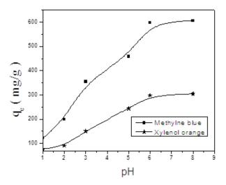
Fig. 8. Effect of pH on the adsorption of dyes by P(PVA-MAAc/ HEMA) at room temperature, composition of PVA: MAAc-HEMA (1:1) at time 1h.
