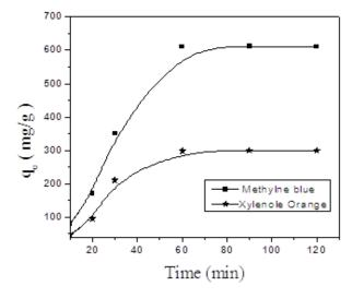
Fig. 7. Effect of time on the adsorption of dyes by P(PVA-MAAc/ HEMA) at room temperature, composition of PVA: MAAc-HEMA (1:1).
