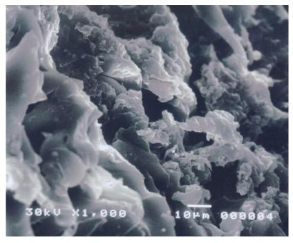
Fig. 3. Scanning electron microscope (SEM) of P(PVA-MAAc/ HEMA). Egypt. J. Rad. Sci. Applic., Vol. 28, No. 1-2 (2015)
