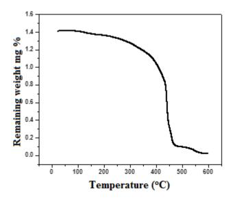
Fig. 5. Thermogravimetric analysis (TGA) of P(PVA-MAAc/ HEMA). *Swelling behaviour*
