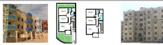
Figure 8, Respectively; Elevation for Ebni Betak scheme in sherouk city, Ground floor plan, First floor plan 75 m<sup>2</sup> unit's area.
