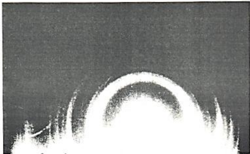
Fig. 1: Electron diffraction pattern of titanium films of thickness 36 nm.
