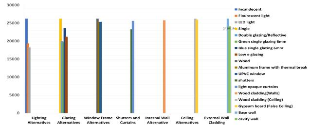
Figure 17, the Annual Energy Consumption (Kwh) for the different retrofit scenarios compared to the base case existing conditions. (Source: The Authors).
