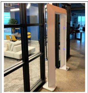
Figure 13, UV-C light system installed office entrance: cbinsights.com, 2020
