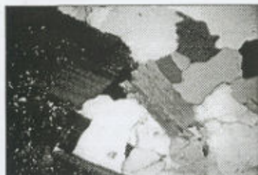
Fig.(8): Quartz , plagioclase , potash feldspar and biotite
