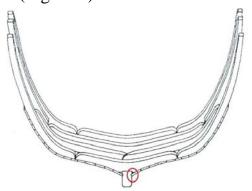
Figure 8: Used of rabbeting planes to make garboard under keel (Doorninck 1976 :118 ,fig 3,4)
