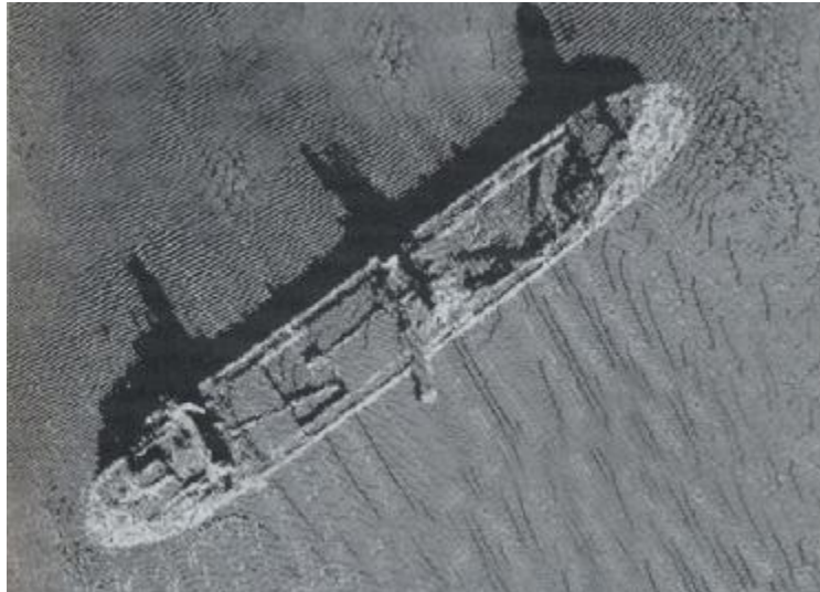
Figure 3: Multibeam image of shipwreck in the Persian Gulf. Data collected by RESON SeaBatMultibeam System (Green, 2004).
