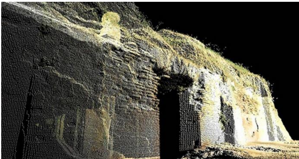
Figure 1: Point cloud laser scan dataset of the cistern complex of Portus, the principal port for the ancient city of Rome( http://www.portusproject.org )
