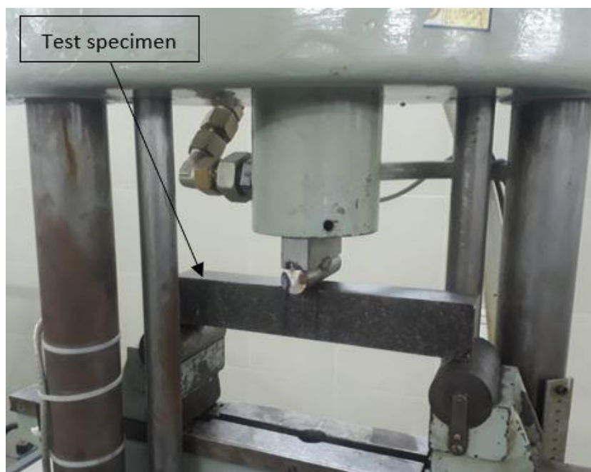
Fig. 6. Flexural test set-up
