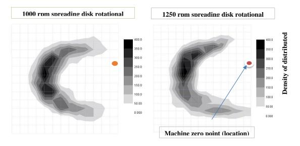
**Fig 6.** 3D visualization of fish feed type 1 distribution pattern and density under 1000 and 1250 rpm spreading disk rotational speed and outlet slide settings 1 (only quarter of the outlet opening)
