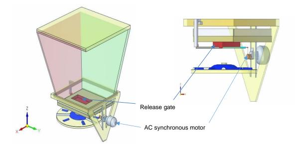
Fig 4. Delivered feed rate mechanism
