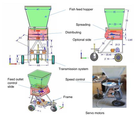
Fig 1. Major components of developed mobile fish feeder
