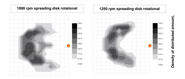
**Fig 9.** 3D visualization of fish feed type 2 distribution pattern and density under 1000 and 1250 rpm spreading disk rotational speed and outlet slide settings 2 (only half of the outlet opening)
