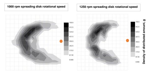
**Fig. 7.** 3D visualization of fish feed type 1 distribution pattern and density under 1000 and 1250 rpm spreading disk rotational speed and outlet slide settings 2 (only half of the outlet opening)
