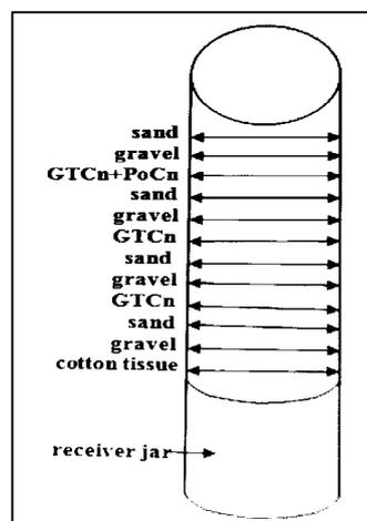
**Fig. 2. A pictorial view of installing a salinity treatment filter from tanneries' industrial effluent**
