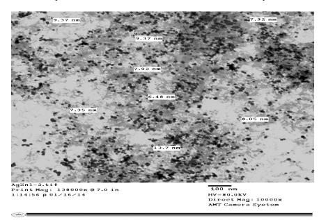
Fig. 2 .TEM image of Ag nanoparticles.
