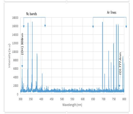
Fig. 2. Emission spectra of Ar plasma jet at 300-800 nm. Applied voltage = 4.5 kV, gas flow rate =4l/m and position of plasma jet = 1 cm.
