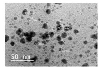
Fig. 1. (b): TEM image of SA/PVP hybrid emulsion loaded with TBHQ.
