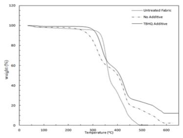
Fig. 2. TGA of untreated and water repellent fabric samples.
