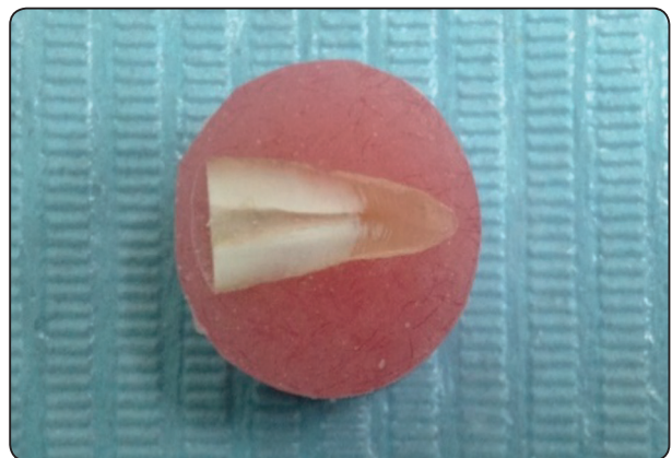
Fig. (1.B) Specimen embedded in auto polymerized resin
