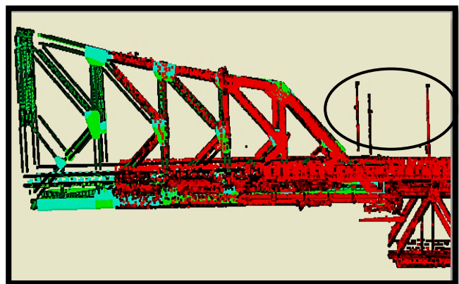
Fig.15. Aligning scanned truss with light columns [red], and designed truss [green] (without light columns).
