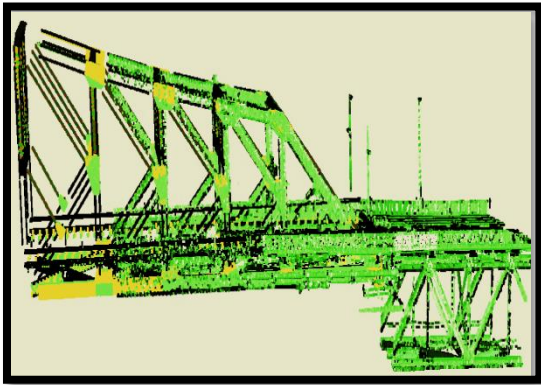
Fig.16. The final result of alignment of the two truss models, standard deviation = 0.12 m.
