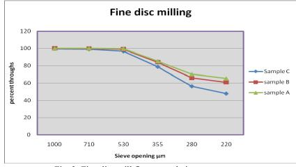
Fig. 2: Fine disc mill flour granulation curve
