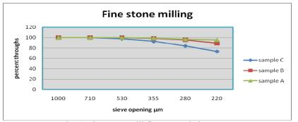
Fig. 1: Fine stone mill flour granulation curve
