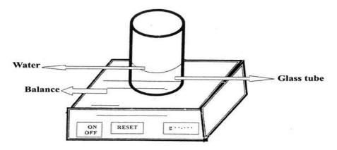
For measuring edema used, a glass open-top cylinder with an internal diameter of 2 cm and height of 5 cm was attached to the center
