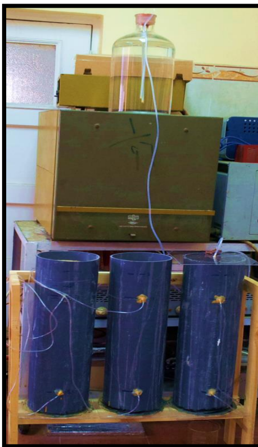
Fig. (1 ). Soil columns experiment layout with Marriott's device for constant water flux
