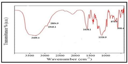
Fig. 1. FTIR spectrum pattern of Nano metal ZnO.
