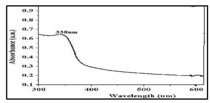
Fig. 3. UV spectroscopy of Nano metal ZnO using Perkin-Elmer S52 Spectrophotometer.
