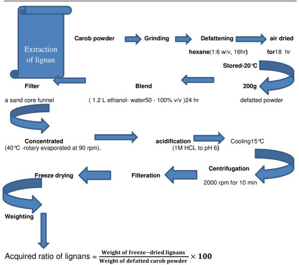
Fig (2). Flow sheet of lignan extraction and determination
