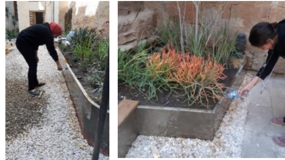
Figure 20: Spraying water to accelerate rusting. [Source: Researchers]
