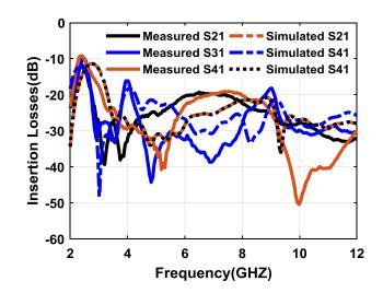
Fig. 14: The measured and simulated insertion of the proposed design.
