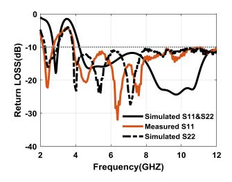
Fig. 13: The measured and simulated return loss of the proposed antenna.
