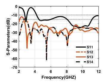
Fig.9: Simulated S-parameters of the proposed antenna.
