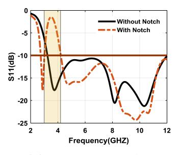
Fig. 2:The simulated return loss results of a singleelement UWB antenna.
