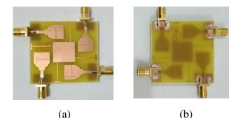
**Fig. 12**: The prototype of the proposed antenna: (a) top layer; (b) the bottom layer.
