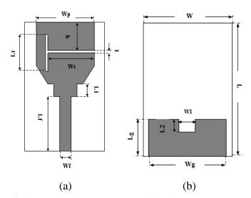
Fig. 1: The proposed antenna layout for a single element: (a) the top layer and (b) the bottom layer.
