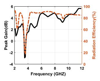
Fig. 11: Simulated realized peak gain and radiation efficiency of the proposed design.
