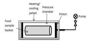
Fig. 1. Diagram showing components of high pressure system.
