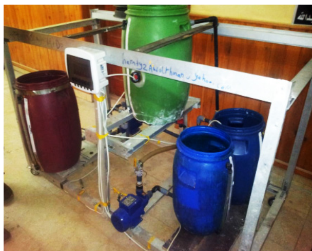
Fig. 3: The assembled constructed biodiesel production unit
