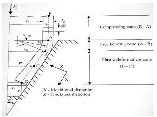
Fig. 1: Nosing die, tube geometry and the coordinate systems Mohammed [18].
