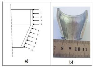
Fig. 19: a) shows the positions of thickness measurements on the nosed part b) photo of the polished sliced part at tube thickness 3.5 mm, semi-die angle 15°, and grease lubricated.
