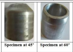
Fig.11 the deformed tubes after nosing process.
