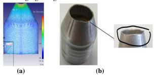
Fig. 23: Earing at conical semi-die angle 15°, wall thickness 1mm and grease-lubricated.
