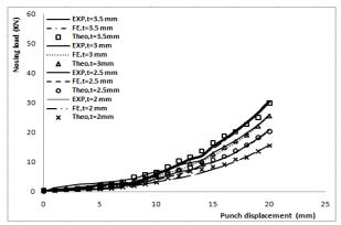
Fig.13 load/ displacement curve in hemispherical die at  $\mu$ =0.04.
