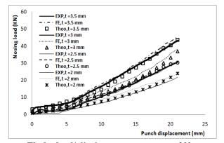
Fig.9c. load/ displacement curve at  $\alpha$ =30°, and  $\mu$ =0.04.
