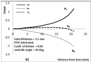
Fig.17. Strain distribution of nosed tube: a)  $\mu = 0.15$ , b)  $\mu = 0.04$ .
