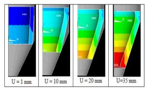
Fig. 16 deformation shape at different die penetration at 15°.
