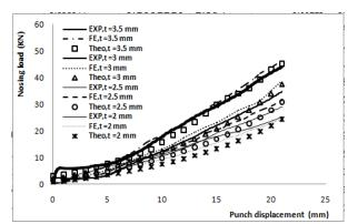
Fig.9b. load/ displacement curve at  $\alpha$ =30°, and  $\mu$ =0.05.
