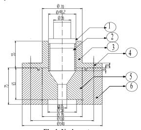
Fig.4: Nosing setup 1-Punch, 2- Specimen, 3- Control sleeve, 4- Bolt (4/90 °), 5- Nosing die, and 6- Die block.
