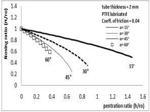
Fig. 15 the relation between nosing ratio (rt / ro) and penetration ratio (h / ro).
