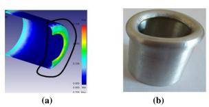
Fig. 21: Folds occurred at conical die with semi-die angle 60° and wall thickness 1.5 mm.
