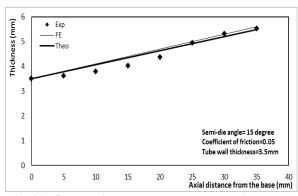
Fig. 20: Correlation between the FE-predicted and the experimentally values of thickness distribution, the values tube thickness 3.5 mm, semi-die angle15°, and grease lubricated.
