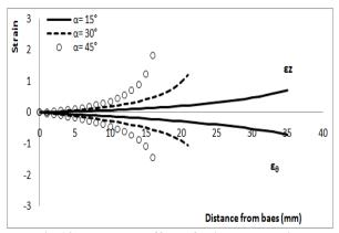
Fig.18. shows the effect of thickness strain distribution at different semi die angle.
