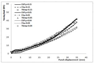
Fig.8: load/ displacement curve at different lubrication condition of the nosing tube.
