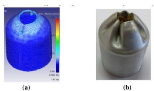
Fig. 22: Wrinkling at conical semi-die angle 45°, wall thickness 1mm and grease-lubricated.
