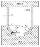
Fig.2: Nosing process using hemispherical die Amirhosseini et al [19].
