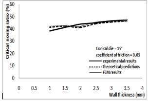
Fig.14: Relationship between wall thickness and critical nosing ratio.
