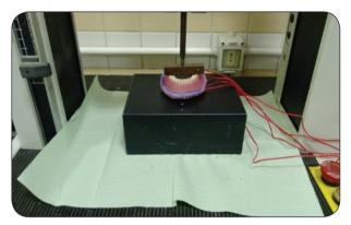
Fig. (1) Bilateral Load application to the acrylic model.
