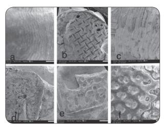
Fig. (6) a) Normal enaml surface. b) Group1, Control group. c) Group2,Cutting bur treatment. d) Group3,Ultra Sonic scaler treatment. e) Group4, Sand blasting treatment. f) Group5,Co<sub>2</sub> laser treatment.
