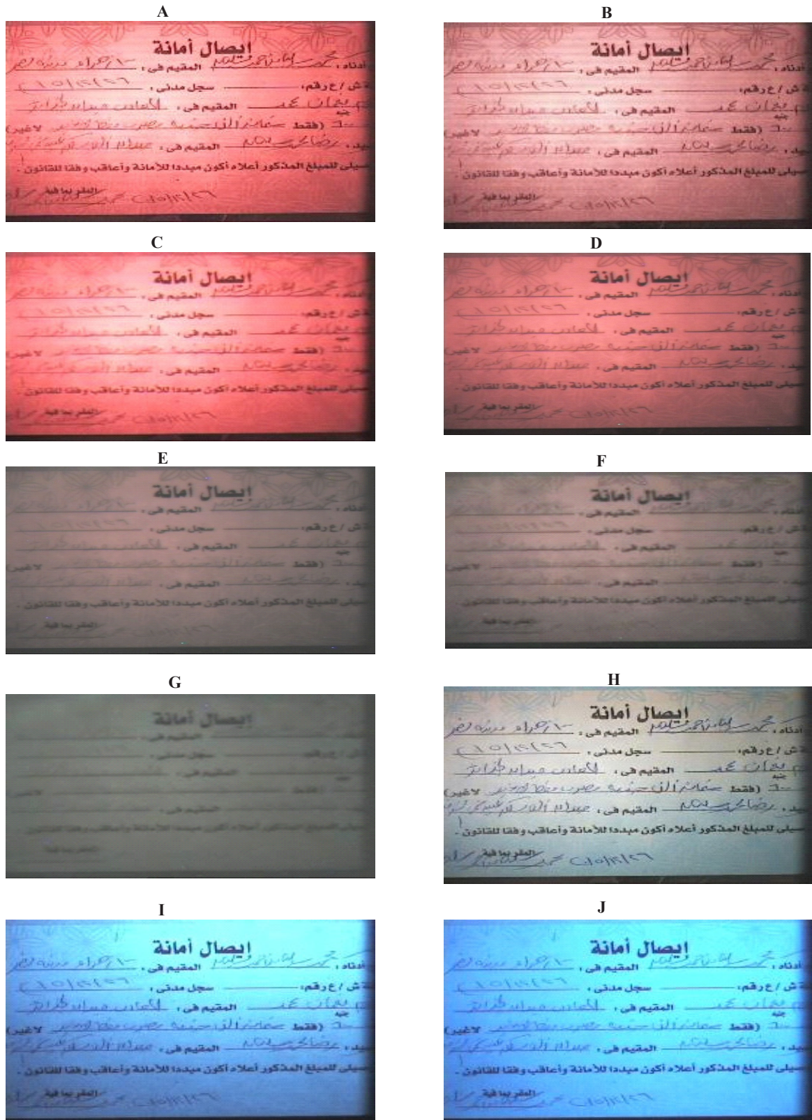
Fig. 8 . The trust receipt which was written with the Bic ballpoint pen under different wavebands where; 630 nm., (B) 645 nm, (C) 665 nm, (D) 695 nm, (E) 715 nm, (F) 735 nm, (G) 780 nm, (H) No filter (I) 254 nm, (J) 365 nm.
