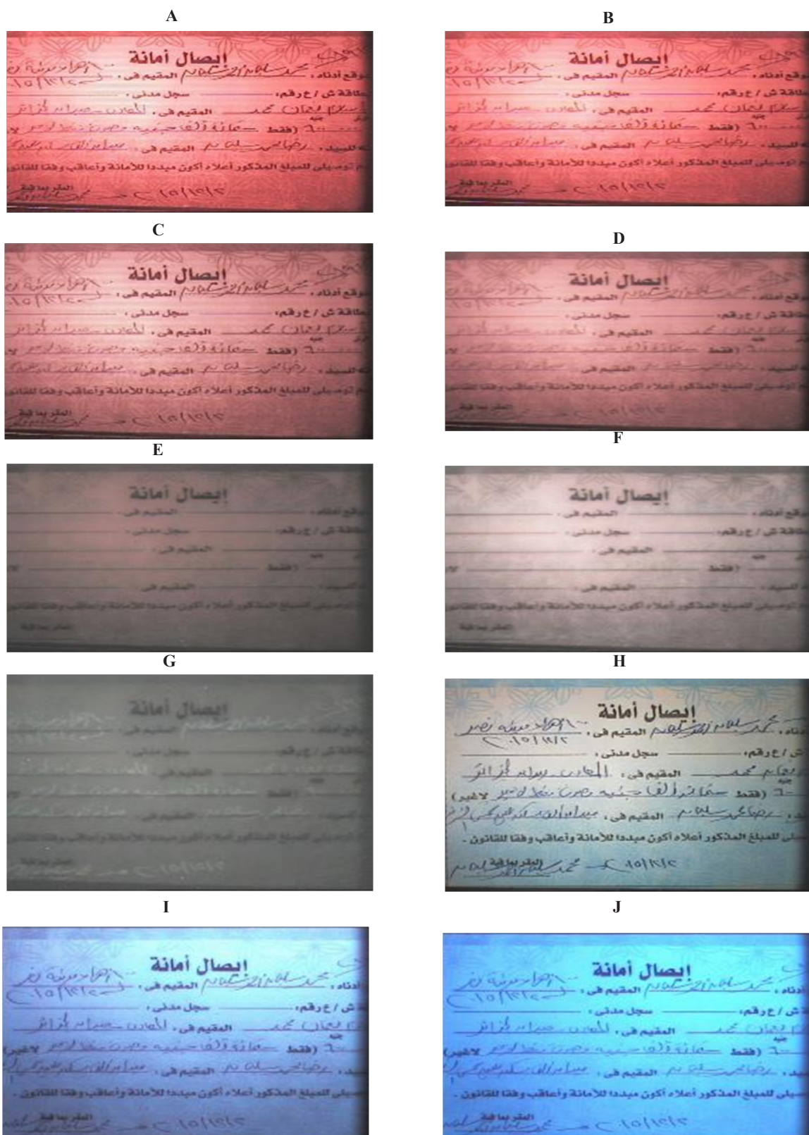
Fig. 9. The trust receipt which was written with the Reynolds ballpoint pen under different wavebands where; (A)630 nm., (B) 645 nm, (C) 665 nm, (D) 695 nm, (E) 715 nm, (F) 735 nm, (G) 780 nm, (H) No filter (I) 254 nm, (J) 365 nm.
