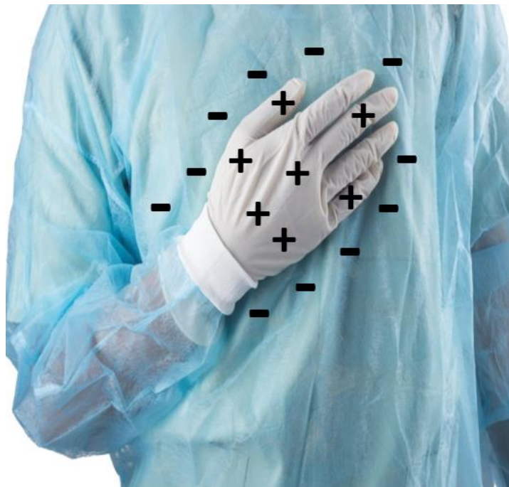
Fig. 8 illustration of the distribution of ESC on the surfaces of gloves and doctor gown.
