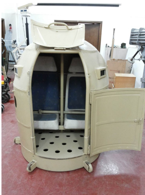
Fig. 8 : (a) Manufactured safety pod main door and hatches
